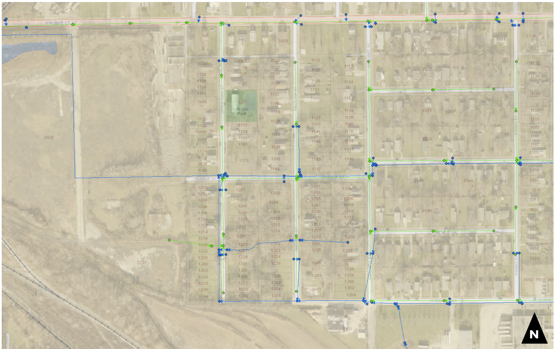
figure 8: Sewer network - storm lines and inlets indicated in blue; sanitary lines and manholes indicated in green
